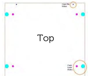
**NOTE:** In the Top and Bottom Panels Insert the cam pins on the opposite side to the Cam Lock.
