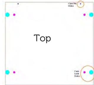
**Cam Pins** Insert all Cam Pins into the following panels as described by the cabinet part located on the cabinet sticker.
